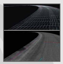
The LDTM data of 1 mm resolution can be imported as .LAS and Bentley MicroStation formatted files for easy use and analysis.
