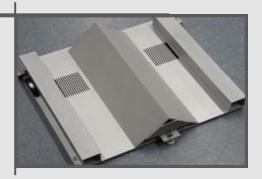
The *LCMS Validation Tool* uses a calibrated pyramidal object along with a test software to validate the calibration of the Sensors. The validation includes:
