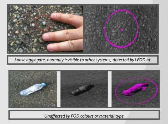
The Laser Foreign Object Debris (LFOD) detection module upgrade uses the dynamic LCMS technology to acquire high resolution 3D profiles of airport runways, taxiways and aprons to detect even the smallest objects at highway speeds.
